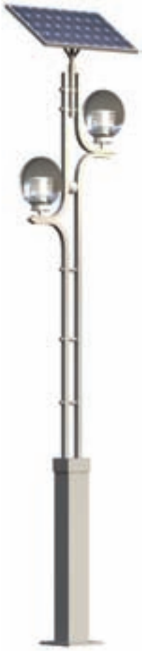
Model Number: EPWL-05 • Power: 65W • Battery: 12V - 65Ah • Height: 3.5m • Light source: 12V/9W x 2
