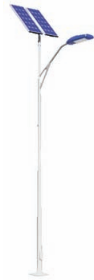
Model Number: EPSL-01L • Power: 55W • Battery: 12V - 50Ah • Height: 5m • Light source: LED 12V/15W
